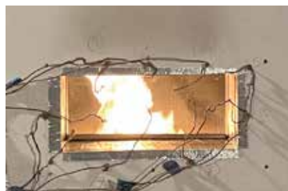
Vent Application testing in progress to achieve compliance to ASTM E2886 Bushfire Mesh TOUGH Shield
