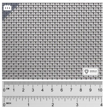
Stock Status Stocked Uncoated **Finish** Mill Finish **Weave Type** Plain Weave Approx Kg/m<sup>2</sup> 3.61 kg/m<sup>2</sup> Approx % Open Area 43 %
