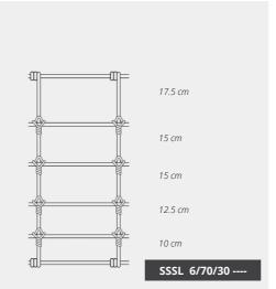
6/70/30 Rolls: 25 m & Fence Picket & Line 100 m 2.50 mm Wire Diam No of Wires 700 mm Fence Height Picket Spacing 300 mm Roll Weight 9.5 kg & 38 Kg
