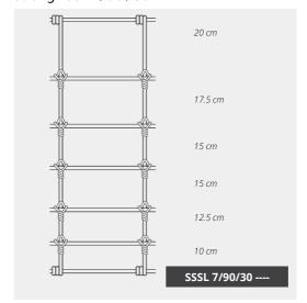
7/90/30 Fence Picket & Line Wire Diam 2.50 mm No of Wires 900 mm Fence Height Picket Spacing 300 mm Roll Weight 11 kg & 45 Kg Grade 316
