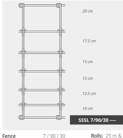
7/90/30 Picket & Line Wire Diam 2.50 mm No of Wires 900 mm Fence Height Picket Spacing 300 mm Roll Weight 11 kg & 45 Kg 316
