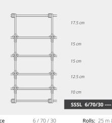
Fence Picket & Line 2.50 mm Wire Diam No of Wires 6 700 mm Fence Height Picket Spacing 300 mm Roll Weight 316 Grade
